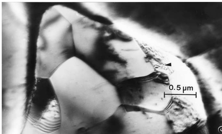
Figure 2 Optical metallographic (a) and TEM ((b) and (c)) views of the starting, Be 62-Al 38 base metal microstructures. (a) Typical microstructure view of Be phase particles in a continuous Al matrix. (b) TEM bright-field image showing the base metal component microstructures. (c) TEM bright-field image showing fine Be grains composing a Be aggregate/agglomerate.
